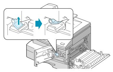
4 Pull the toner cartridge out and gently shake the cartridge to distribute the toner evenly inside the cartridge.
